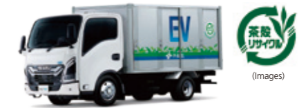
Industry-first EV Bottle Car (with used tea leaf lightweight panels) (Introduced in October 2023)
