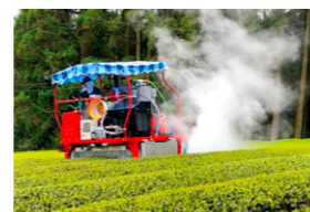
Developing a steam weed control/weeding machine that can control and remove weeds without using pesticides to promote reduced pesticide use and organic cultivation
