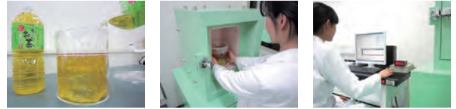
A view of a radioactive substance test using a germanium semiconductor detector. A germanium semiconductor detector is used for testing foods whose standard value is 10Bq/kg or below or 50Bq/kg or below, including beverages, tea for drinking (extracted liquids), water used in such products, milk and milk-based drinks.
